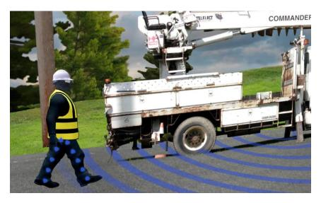
If a boom truck contacts an energized conductor, it can create deadly touch and step potentials. Rubber gloves or insulated footwear can protect you. Grounding the truck to the neutral reduces these hazards.
