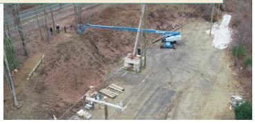
In some cases, utilities must place all three phases on the crossarm. Full-scale testing showed that the utility could expect all three phases to break away from the crossarm, but the pole remained undamaged. 'Saving the pole' is a design priority when trying to improve storm restoration times.
