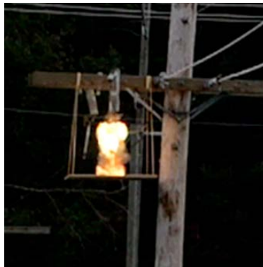
Figure 13. Fuse fireball attempting to ignite shredded wood fibers
