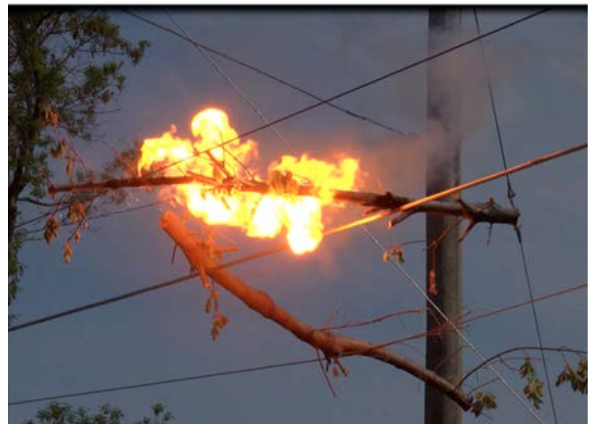
Figure 5. Limb across 12 kV conductors developing into a high-current fault
