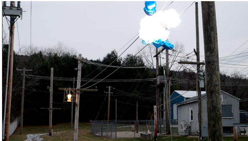
Figure 12. Fuse operating to clear an arc across a mylar balloon
