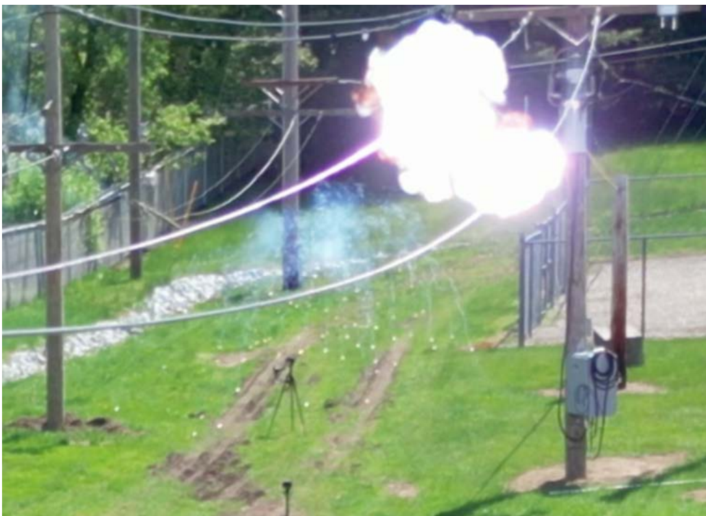
Figure 1. Arc and molten metal from conductor slap
