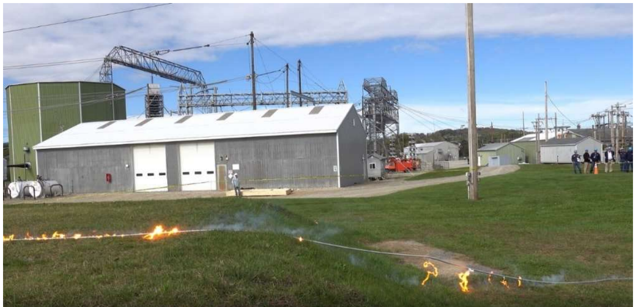
Figure 7.2 Arcing to Ground Vegetation from a Live Downed Conductor Test
