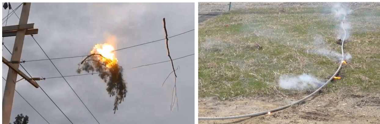
Figure 7.4 Different Ignition Sources from Contact with Vegetation
