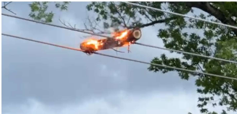
Figure A.2 Tree limb burning together from each end (EPRI workshop, 2022)
