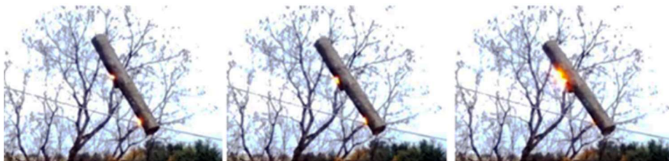
Figure A-6 Tree limb burning across #4 copper wire due to localized heating prior to a high-current fault [2]
