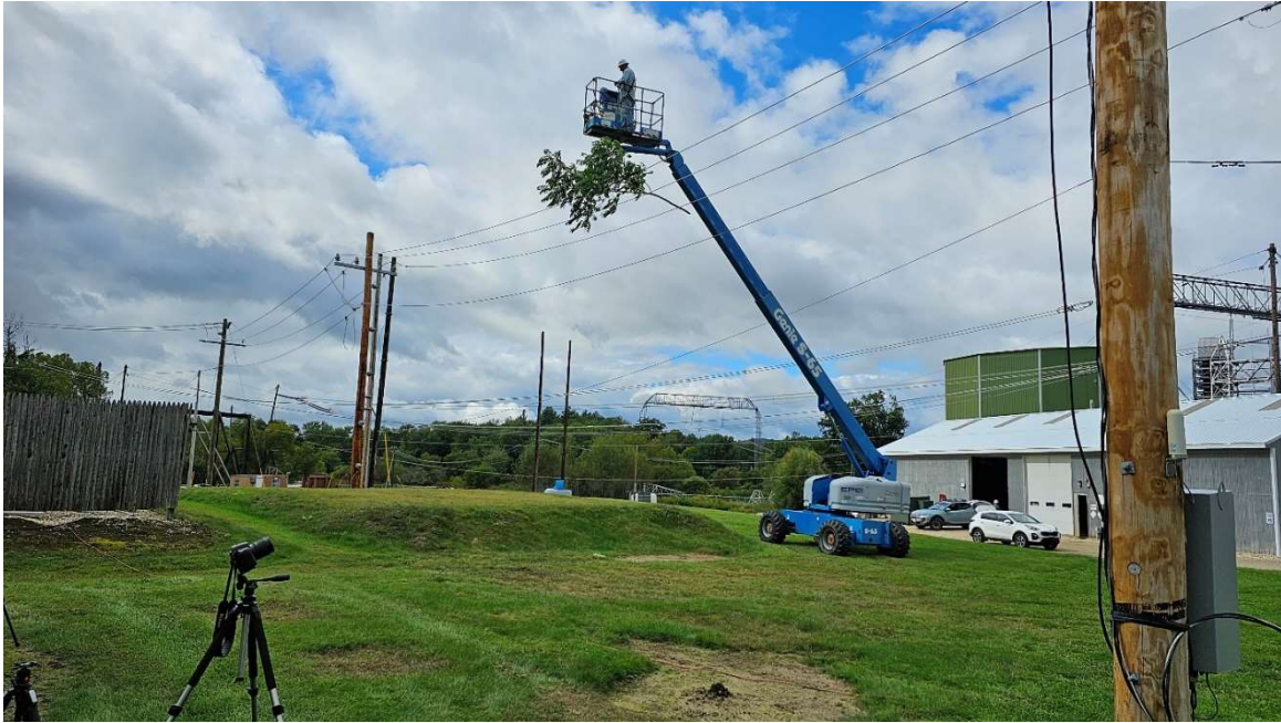
Figure B.2 Vegetation drop tests on de-energized three-phase line
