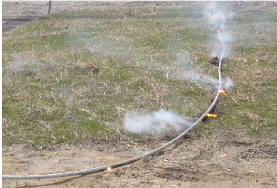
Figure A.5 Energized downed conductor [1]
