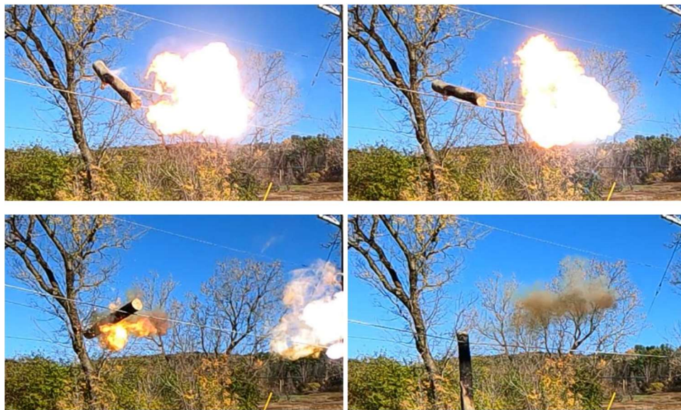
Figure A.7 Wire Burndown – resulting in a live downed conductor [2]
