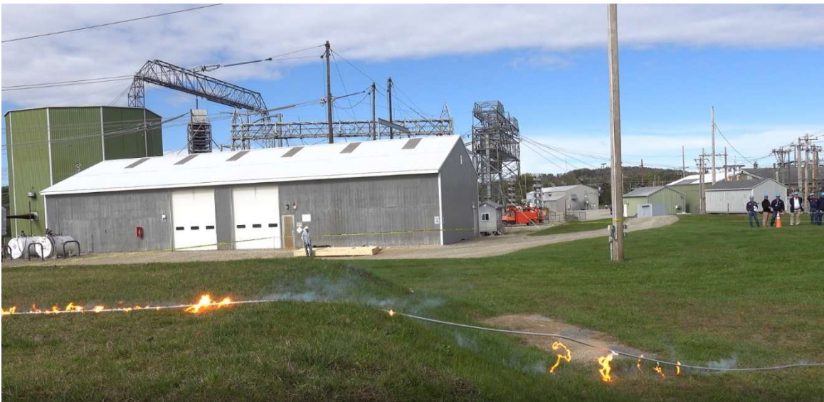
Figure B.3 Energized 13.2/23kV bare conductor break onto grass
