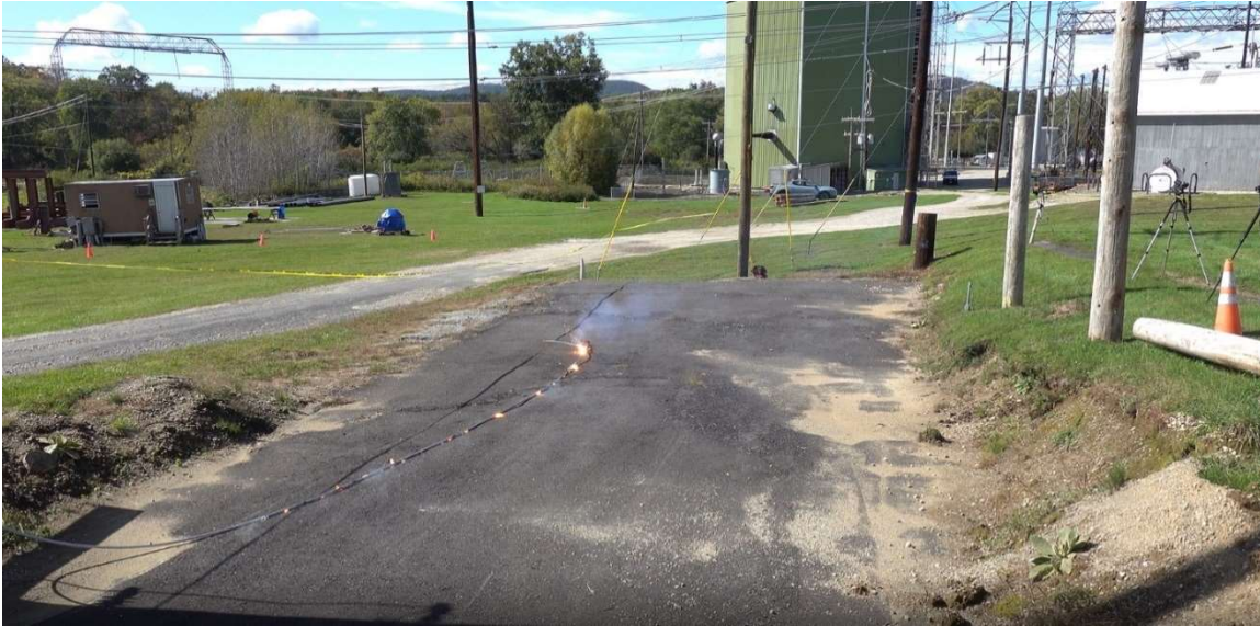
Figure B.4 Energized 13.2/23kV and 7.2/12.47kV bare conductor breaks onto asphalt
